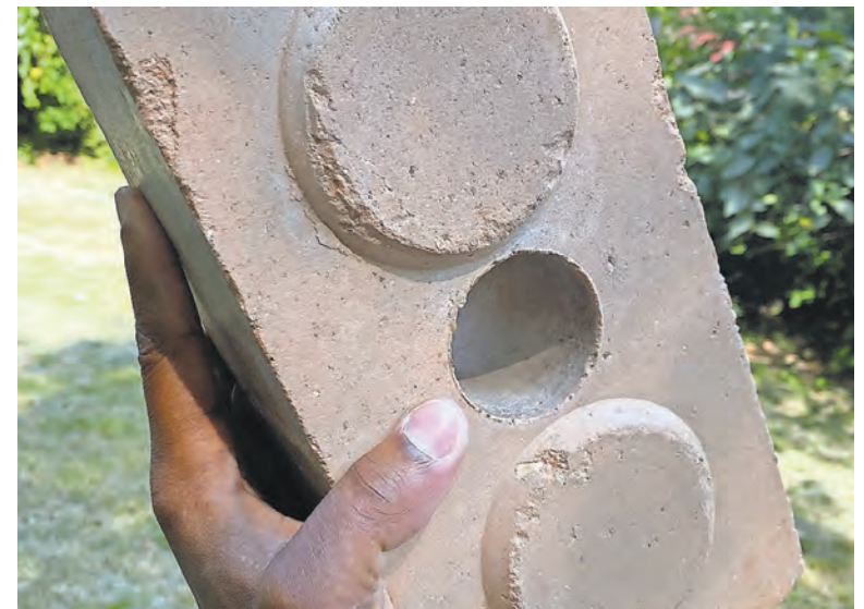
CEB bricks are made by compressing a mixture of soil, water and cement into oversized earth bricks.
